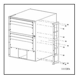
2 Insert and tighten the supplied flat-head screws to fasten each bracket to the chassis.
